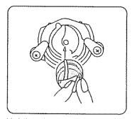
case into shuttle and release when latch is released. latch.
